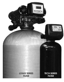
SWT's Commercial Iron, Hydrogen Sulfide, and Manganese Filters are built utilizing SWT's MetalEase filtration media. These chemical-free filters are designed to remove metals along with sediment and turbidity from water. Vigorous backwashing keeps the bed clean. SWT takes care of the little extras such as machined PVC distribution systems and garnet underbedding to prevent channeling.
